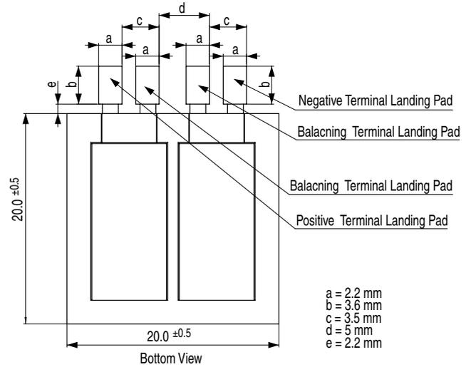
Soldering pads to Case TS20, TS22, TS32, TS35, FS37
