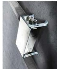
MULTIBOX UPB The MULTIBOX UPB can be set in concrete directly with the simplest means. The UPB version is mounted on the formwork in a few easy steps and adjusted to the wall thickness with the wing screws.
