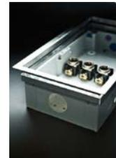
MULTIBOX UPB After the pipes have been installed, the MULTIBOX can be set in concrete. As soon as the formwork is stripped, the polystyrene block is removed and the safety elements are installed and connected. The front frame and the cover form the end.
