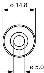
Cable diameter max. 5.0 mm
