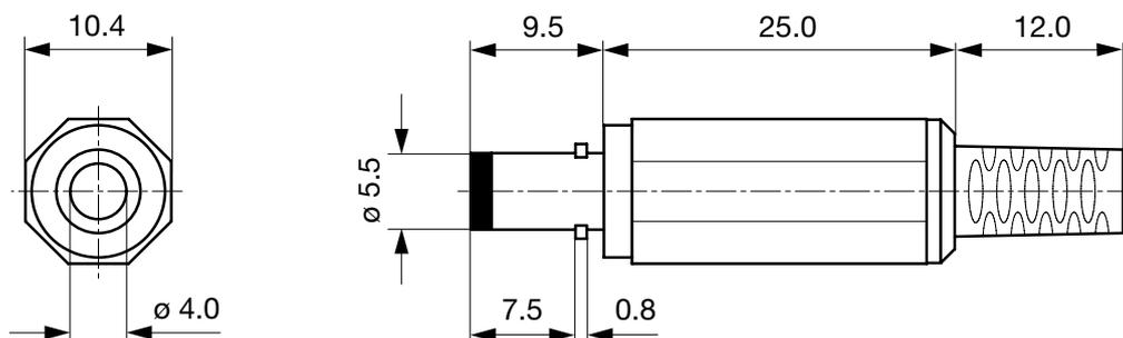
Cable diameter max. 4.0 mm
