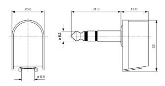
Cable diameter max. 8.0 mm
