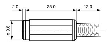
Cable diameter max. 4.0 mm
