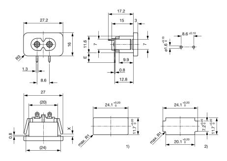
E = PCB terminal standard (additional solder): 6.8 mm
