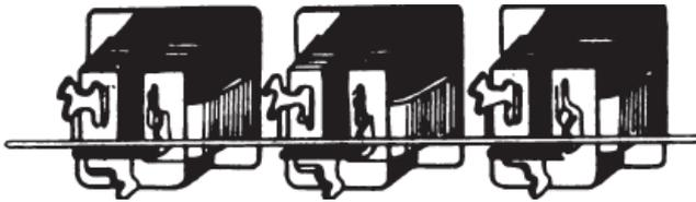
Installation Diagram: V-slotted terminals for connecting multiple receptacles (only for solid bare wires from type 14 AWG)
