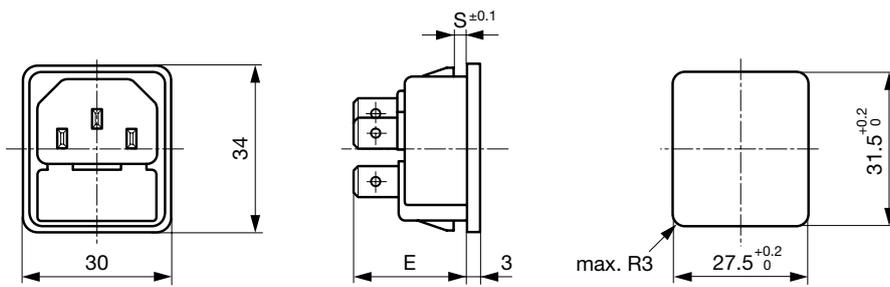
E: Lötanschlüsse 22.5 mm
