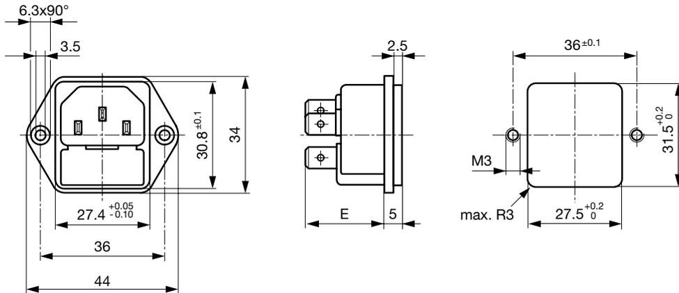
E: Lötanschlüsse 20.5 mm
