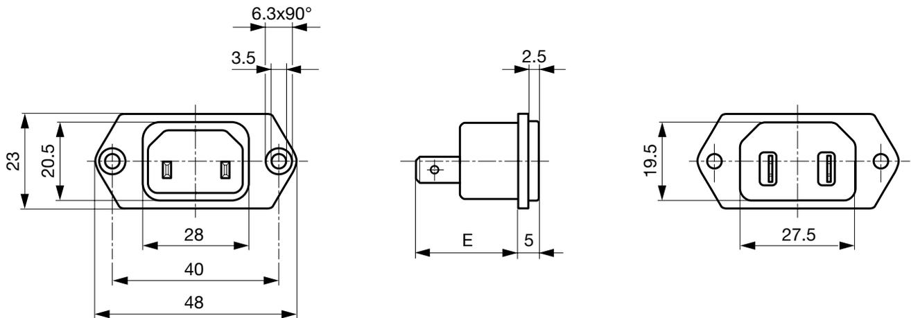
E: Lötanschlüsse 20.5 mm
