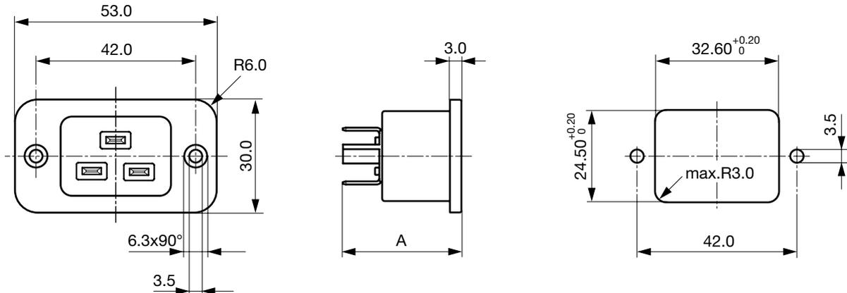
A = 32.0 mm: Steckanschlüsse 6.3 x 0.8 mm
