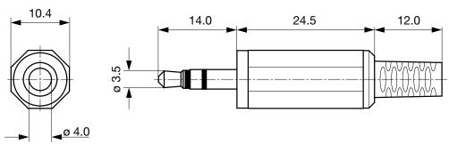
Cable diameter max. 4.0 mm
