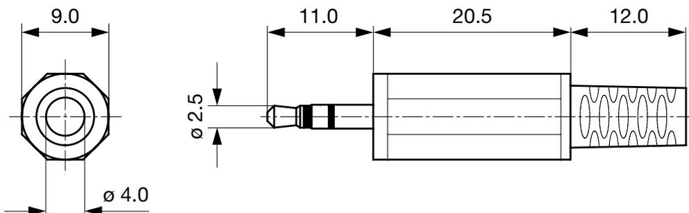
Cable diameter max. 4.0 mm
