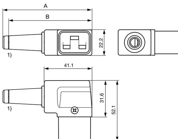
1) Cut strain relief 8 (10) mm here for 10 mm cable
